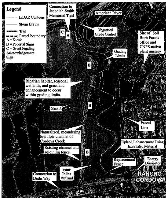
The graphic shows a sinusoidal creek alignment for conceptual interpretation purposes only. The actual alignment will be designed with a more natural perspective.
